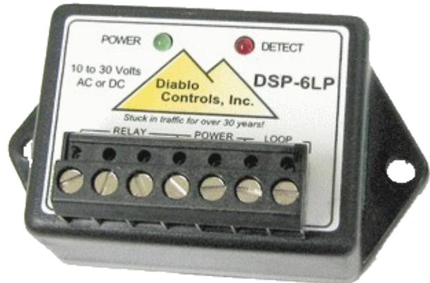
**Power** - 10 to 30 Volts AC or DC. Approximately 1 mA (no car and all loop sizes) and less than 25 mA with a car on the loop.
